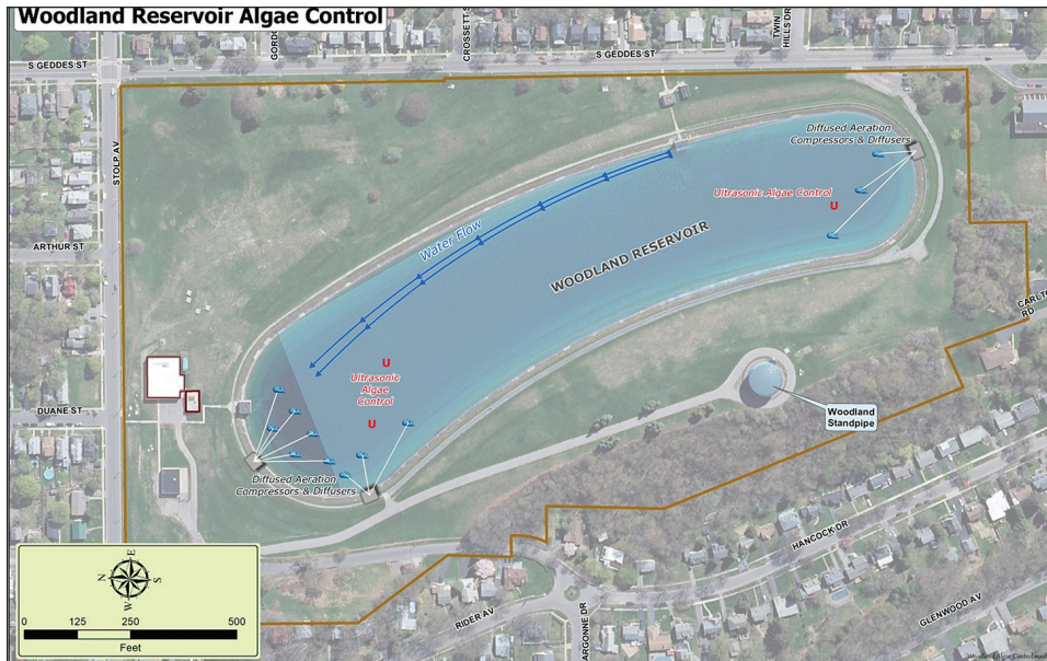
Figure 4. Orthomography of Woodland Reservoir showing algal control stations.
